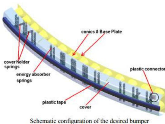
Automotive bumper system plays an important role not only in absorbing impact energy but also in a styling stand point. A great deal of attention with in the automotive industry has been focused upon light weight and sufficient safety in recent years. Therefore, the bumper system equipped with thermoplastic and energy absorbing element is a new world trend in the market. The
