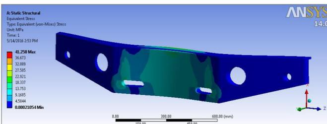
Comparing the both designs, second material design (optimized) is absorbing more loads because of bumper with removed material. And as per the assumed material for beam, stresses are near to yield. Polyethylene has good chemical resistance. Two types are used; low density polyethylene (LDPE) and high density polyethylene (HDPE) can be manufactured in a range of densities. Application: glass reinforced for car bodies, electrical insulation, packaging, where strength and aesthetics are important.
