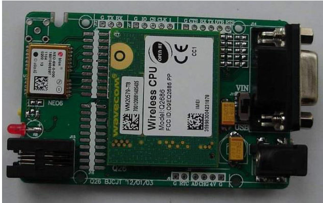
Fig. 2 Q2686 development board.
